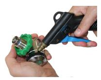
Blow out remaining humidity from the pressure reducer with an air gun. Blow out pressure reducer via ventilation bore holes. Use compressed air with breathing air quality according to EN 12021. One of the bore holes has to show downwards. Blow out in-depth and dry completely.
